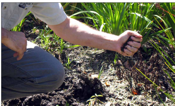
Compressing soil into a ball.
